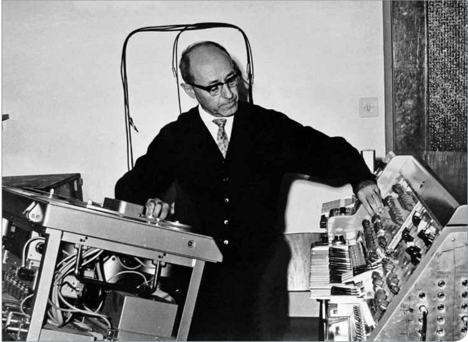
Figure 1. The Israeli composer Josef Tal at the Electronic Music Studio in Jerusalem (~1965). The composer is also the performer (a Hugh Le Caine synthesizer, at right) of the completed product, usually recorded on magnetic tape (a Studer C37 recorder, at left)
